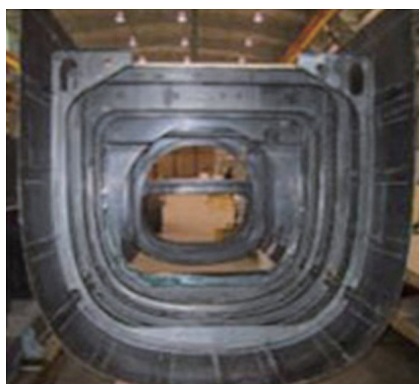
图5 VARI成型的阿帕奇直升机机舱 Fig.5 VARI molding Apache helicopter cabin
