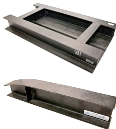
图7 SQRTM成型的复合材料起落架舱 Fig.7 SQRTM molding composite gear compartment
